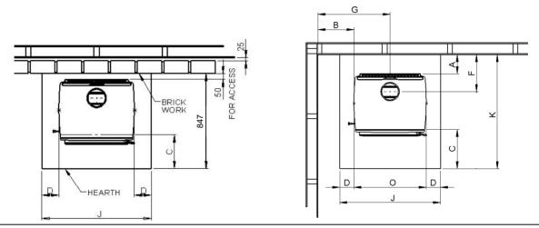
**Above: Non combustible wall clearances.** Brick lining. From the floor to within 25mm of ceiling. Leave air vents at the bottom to allow airflow in the cavity. If Yunca flue mounted shield is fitted, brickwork may be 1200mm high as long as all vertical joints in top and bottom of brickwork are left out to allow airflow when brickwork is capped.
